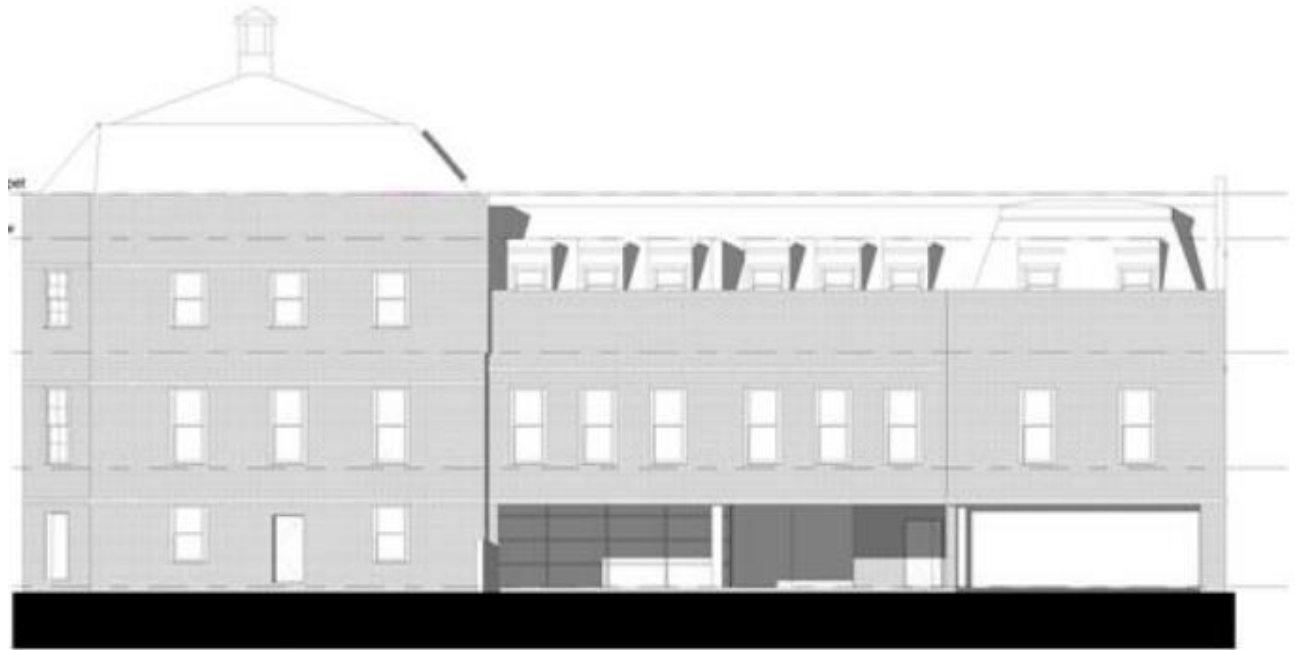
1 Existing North West Elevation 1:100
